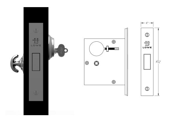
The Lowe 953 full mortise auxiliary deadbolt is available in 2–1/2", 2–3/4", 3–3/4", 5", or 6" backsets. The 953 can be used as an additional auxiliary deadbolt on exterior doors where additional security is desired, or on interior doors for both privacy and security. The lock can be configured to work with mortise cylinders, thumbturns, or emergency release trim. It is supplied with a strikeplate and stamped metal dustbox, and the faceplate has an adjustable bevel.
