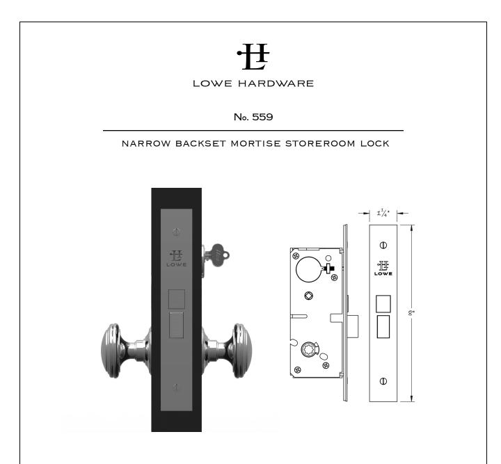
The Lowe 559 light duty, narrow backset mortise storeroom lock is available with a 1–1/4" backset. Typically used as a storeroom lock, from the outside the 559 maintains a locked position always requiring a key to enter. From the inside free egress is always available. It is supplied with a strikeplate and stamped metal dustbox, and the faceplate has an adjustable bevel. The 559 is also available for use upside down. Available in any of our yacht quality finishes.
