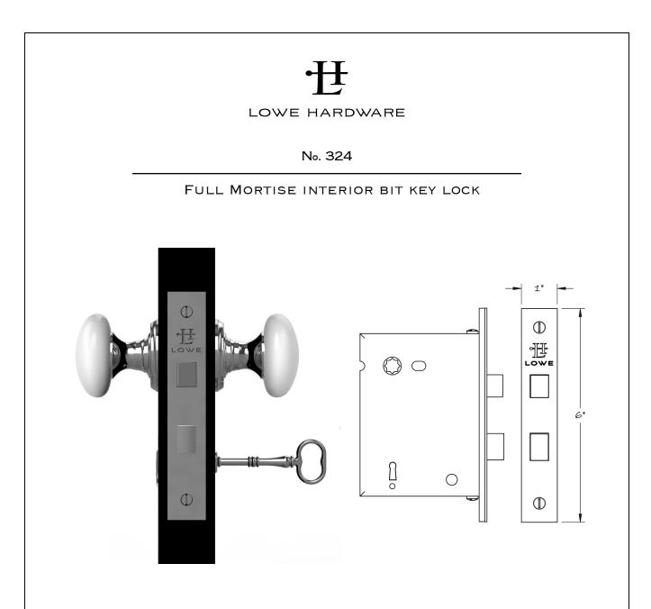
The Lowe 324 full mortise interior bit key lock is available in 2–1/2" or 2–3/4" backsets. The 324 is typically used on interior privacy doors of all sizes where the use of a bit key is desired. The lock can be configured at the factory to be used with knobs or levers. It is supplied with a strikeplate and stamped metal dustbox, and the faceplate has an adjustable bevel. Spacing between the handle and bit key is 2–7/8". Available in any of our yacht quality finishes.
