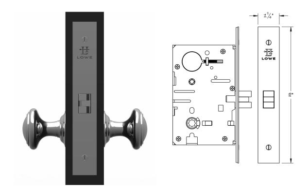
The Lowe 125 full mortise passage lock is available in 2–1/2", 2–3/4", 3–3/4", 5" or 6" backsets. The 125 is typically used on passage doors that require a listed lockset. The lock can be configured at the factory to be used with knobs, levers, thumblatches or any combination thereof. It is supplied with a strikeplate and stamped metal dustbox, and the faceplate has an adjustable bevel. The 125 is ANSI Grade 1, and is UL listed with a 3 hour fire rating.
