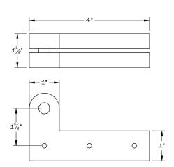
The Lowe 8000 T1,D1 offset pivot hinge is shown here with a 1.25" offset.
